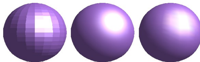
Figure 25: Flat, Phong and Gouraud shading
