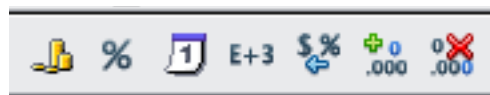
Figure 30: Number format icons. Left to right: currency, percentage, date, exponential, standard, add decimal place, delete decimal place.
