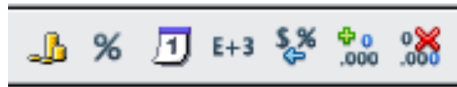
Figure 95: Number format icons. Left to right: currency, percentage, date, exponential, standard, add decimal place, delete decimal place.
