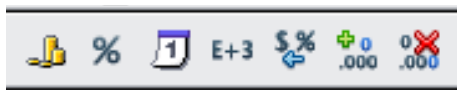
Figure 31: Number format icons. Left to right: currency, percentage, date, exponential, standard, add decimal place, delete decimal place.
